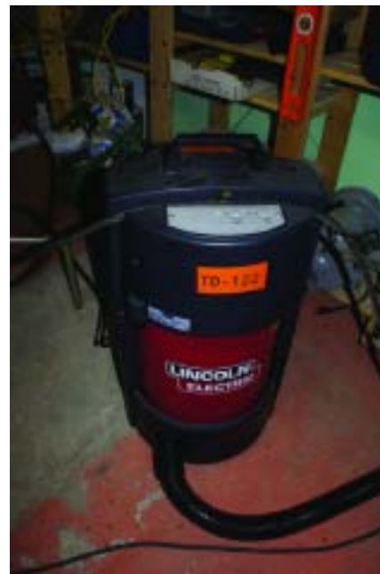
The Miniflex with the welder's lead mounted for automatic operation.
