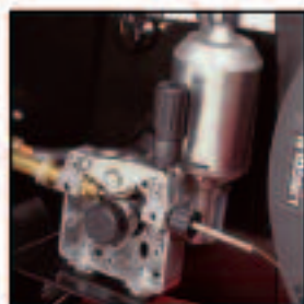
Integrated REDI-MIG's feature a 2 drive roll system
